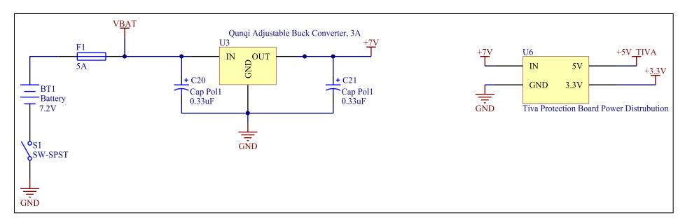
No actuators in the FARMER, and the current draw is not remotely close to 3A.
