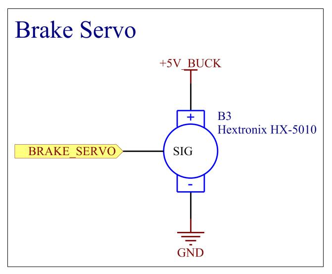
This servo normally takes less than 0.25 A, which is well within the capability (3A) of the buck converter.
