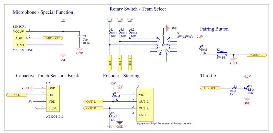
Tiva is 5V tolerant, so it's fine to use these 5V sensors' outputs.
